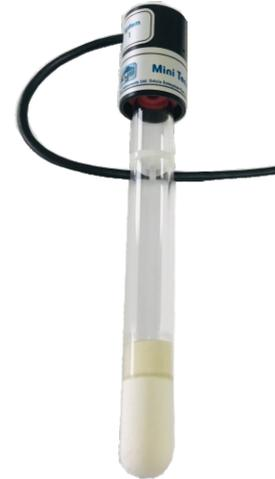
Small design allows insertion into soil without damaging nearby plant roots
