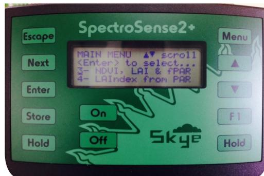
Logging display meter for visible/NIR light sensors
