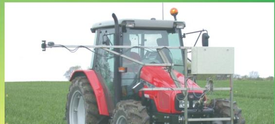
2 x 4 band Skye radiometers measuring the incident & reflected light
