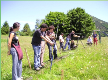
Comparing broadband NDVI against spectroradiometer measurements
