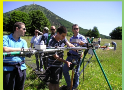
Comparing hand held NDVI against Flux Tower measurements
