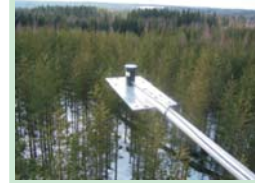
Skye 2-channel sensors on an Eddy-Covariance Tower. Courtesy: Dr. Caroline Nichol
