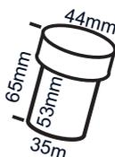
Mounting - M6 x 7mm tapped hole in base. Sensor supplied with M6 x 16mm screw + 4x 1.5mm washers to suit panel thicknesses of 3-10mm
